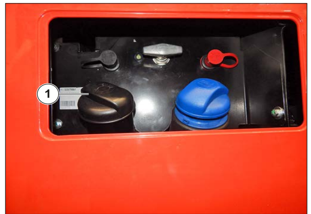
Figure 121: Filling the fuel tank
