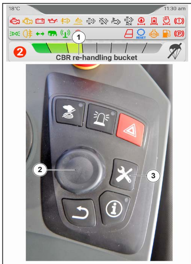
Figure 125: Selection and confirmation of attachment
