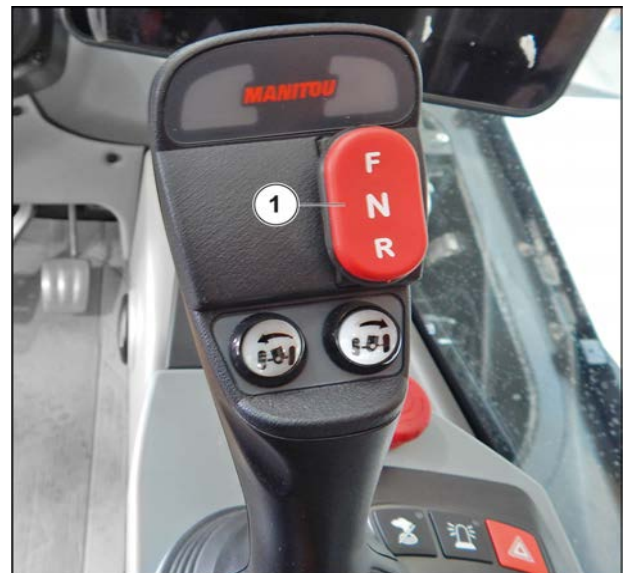
Figure 132: Using the FNR selector
