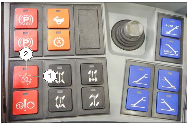
Figure 133: Travel safety system reset button
