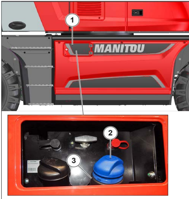
Figure 149: Checking DEF liquid level
