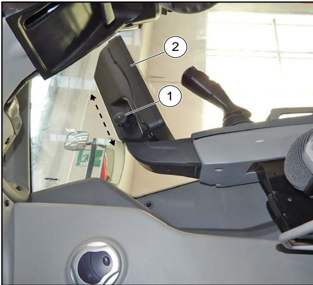
Figure 56: Display height adjustment knob
